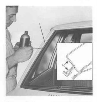
Degrease the inner perimeter of the glass, using cotton wool soaked in methylethyl alcohol.
