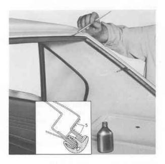
Degrease the inside perimeter of the rear screen with cotton wool soaked in methylethyl alcohol.
