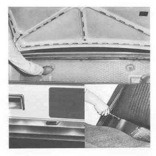
Lift padded Texalfa strip, unscrew the three screws fixing the rear shelf and remove the shelf.
