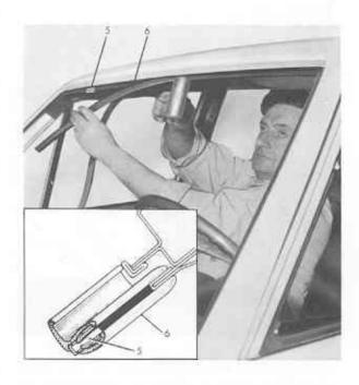
Fit trim 7 to the two windscreen pillars and secure with screws.
