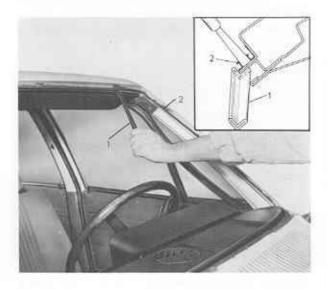
Brush the recommended Primer to the groove of the new windscreen space moulding and to the corresponding areas of the metal surface of the pillars and to the header panel. After the Primer has set, fit moulding 3 to the edges in the aperture.
