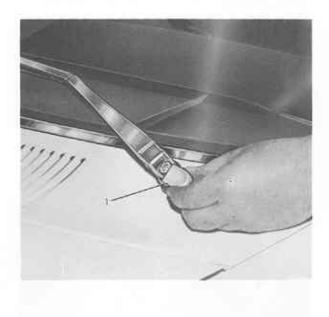
Insert tool no. 2 (A. 9.0064) near one of the corners of the windscreen. Raise the finisher 3 and unhook it from the retaining clips 4. Remove joint cover 5 from the finishers. Repeat this operation along the entire perimeter of the finisher until it is completely detached.
