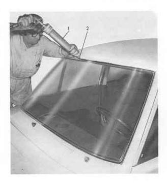
finisher to the adhesive bead, and arrange as shown at illustration on page 5.
